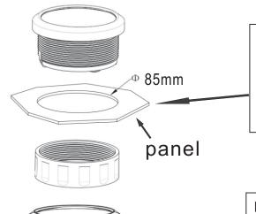
Before installation, firstly, to open a hole Ф85mm of the panel ,make sure there is a space with (55mm backyard of panel)as well.
